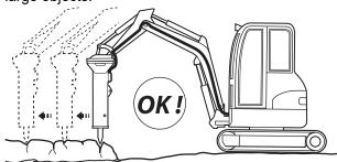
Never run the hydraulic breaker longer then 15 seconds on the same spot. Move the working tool to a new position if the object does not break.
