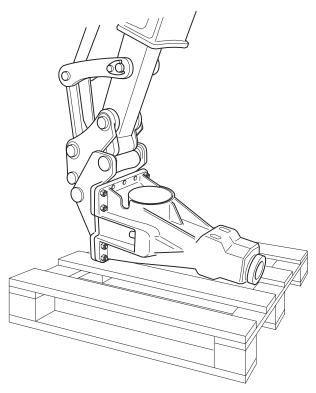
The pressure port on the hydraulic breaker is on the left side when facing the accumulator. If the pressure hose is on the other side of the dipper arm, cross the hoses or turn the hydraulic breaker around.
