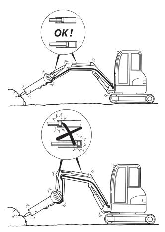
Avoid idling strokes; it causes wear on both working tool and tool retainers.
